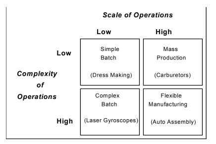
Figure 1 - Characteristics of Process Technology
